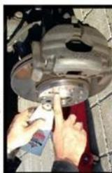
*Place the wheel spacer on the vehicle hub, and then also apply a thin layer of corrosion protection paste to the centering flange on the spacer.*
