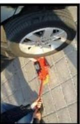
*Raise the vehicle enough to remove the axle stands, then slowly lower the lifting jack.*
