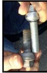
Check, if the length and type of seating of the new and longer bolts are correct. (Have a look overleaf at the bolts advice. The new fixings need to be as long as the originals plus the thickness of the spacer.
