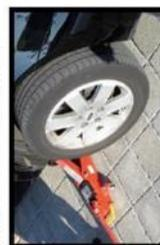
Lift the vehicle until the tire is off the ground, then place an axle stand under the vehicle.
